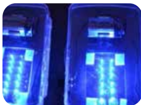
Printed Silver Conductors Powering LEDs
